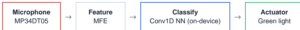
Figure 2.1 Block diagram of the edge processing chain, from audio acquisition to traffic-light actuation.
